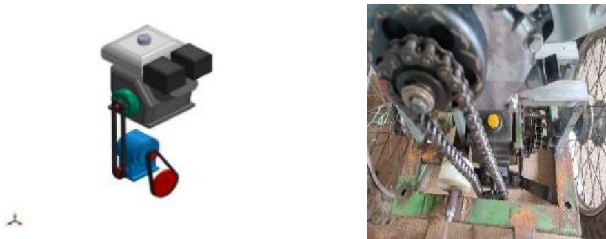
Figure 13. Clutch Transmission Design and Clutch Transmission in Tools.
