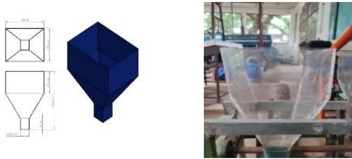
Figure 11. Hopper and Hopper Design on Tools.
