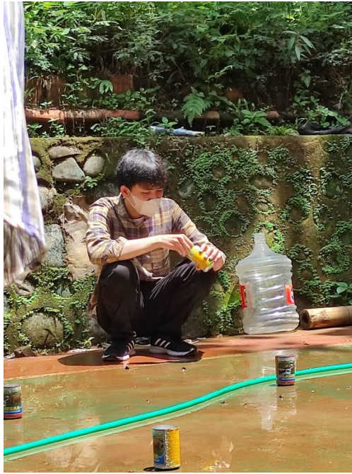
Figure 27. Measuring the discharge of water in a can
