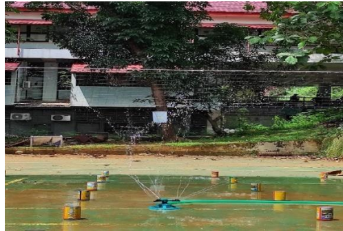
Figure 23. Distribution of 360 sprinkler water
