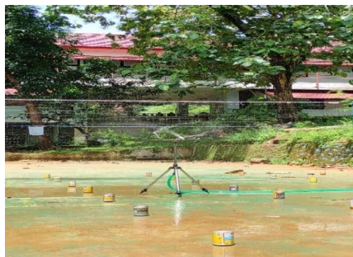
Figure 25. Distribution of 3 nozzle sprinkler water
