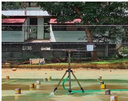
Figure 24. Distribution of 2 nozzle sprinkler water
