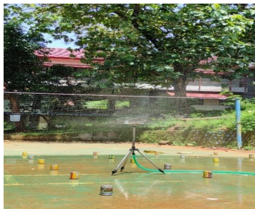
Figure 26. Distribution of 4-nozzle sprinkler water
