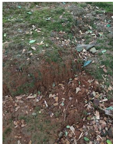
Figure 1. Soil Subject to Groove Erosion.
