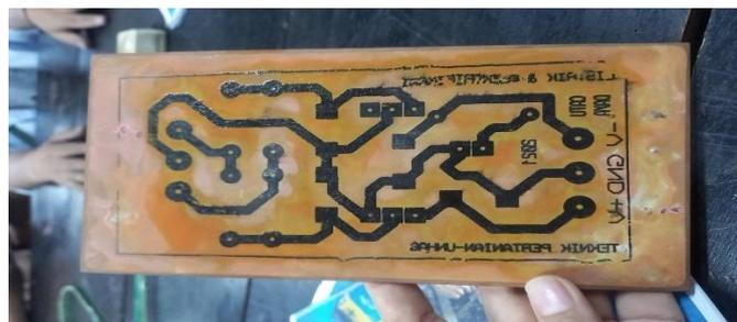
Figure 7. PCB Board Circuit Path.
