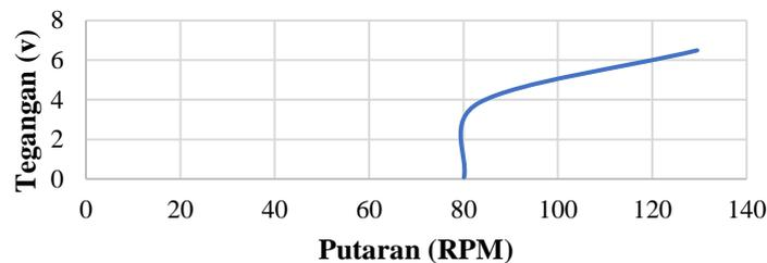
Figure 3. Graph of the Relationship between Voltage (V) and Rotation (RPM).
