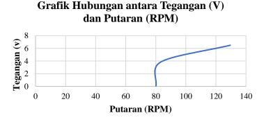
Figure 3. Graph of the Relationship between Voltage (V) and Rotation (RPM).
