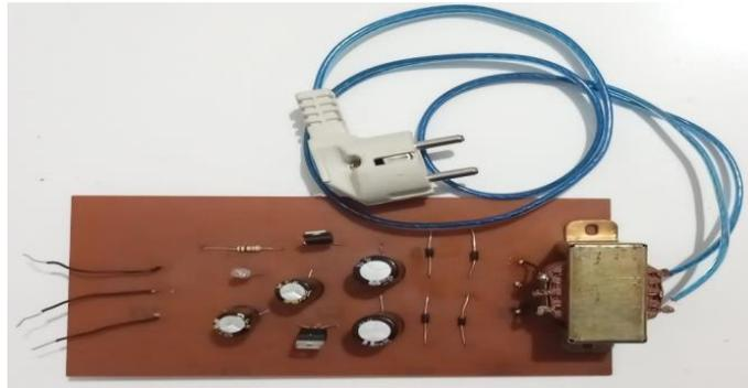
Figure 8. Power supply circuit.
