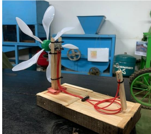
Figure 22. Miniature Hydroelectric Power Plant (PLTA).
