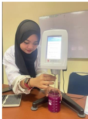
Picture 21. Documentation of Installing Spindle L2.
