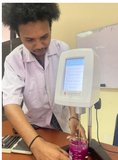
Picture 24. Documentation of Installing Spindle L2.
